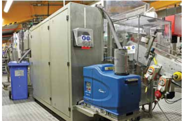
ProBlue Fulfill system with adhesive bin transfer hoses and melter on case packer.
