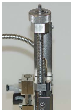
Hand wheel allows easy adjustment of coating width
