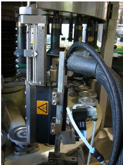
Scale allows precise readout for consistent adhesive deposition.
