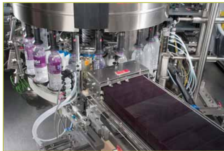
The Nordson non-contact labeling system with PatternJet guns replaces traditional open wheel pot systems in magazine, roll-fed, carousel and in-line labeling application systems.
