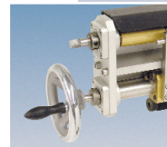
Handwheel for continuous width adjustment from left or right side.
