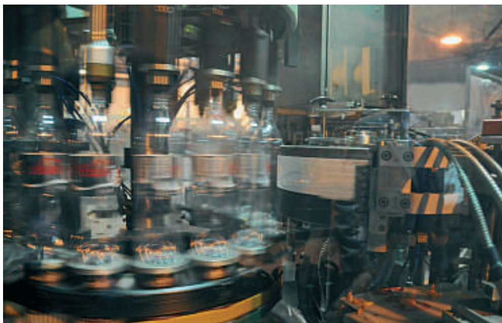
The labeling stations typically run in production with a speed of 24,000 and 20,000 bottles per hour respectively.
