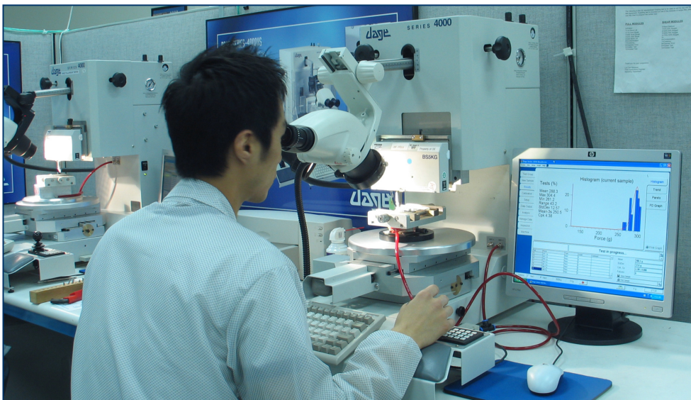
Dage 4000 bond tester performing a wire shear test.
