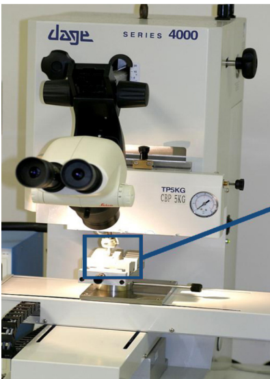
Dage 4000 bond tester performing a cold bump pull test.
