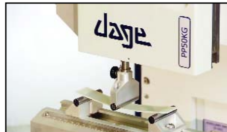
Glass fiber composite undergoing a 3-pt. bend test to assess rigidity and flexural strength.
