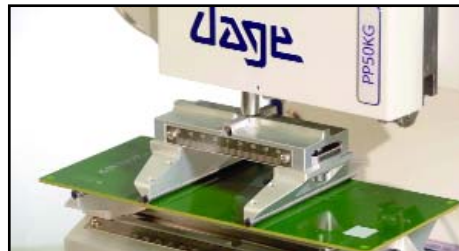
Straining board interconnect using 4-pt. bend.
