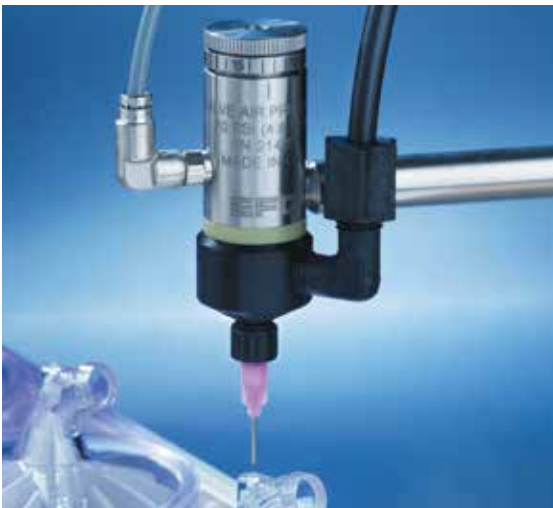
A 752 valve applies UV-cure adhesive to a medical pump.
