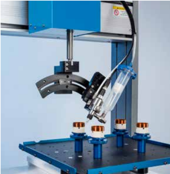
An R Series robot dispenses a rotating circle of material.
