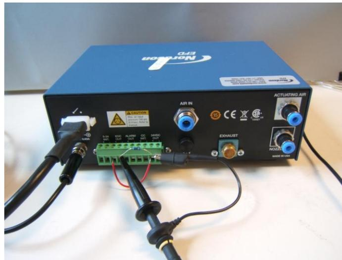
Figure 1: Timer Accuracy Oscilloscope Connection
