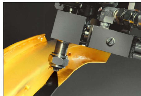
The Flow Coat System applies primer in a non-atomized film pattern
