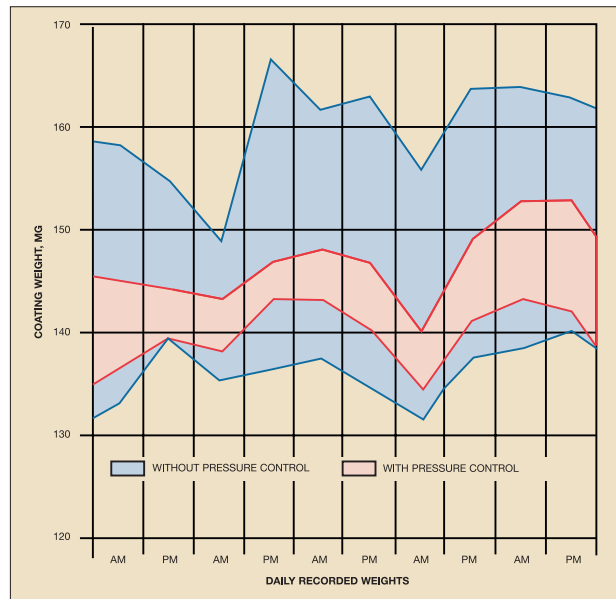
Actual coating weight ranges with and without pressure control.
