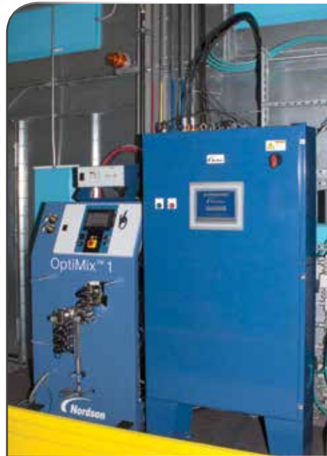
Nordson’s OptiMix 1 plural-component mixing system provides electronically controlled proportioning and mixing of solvent- and water-based coatings.
