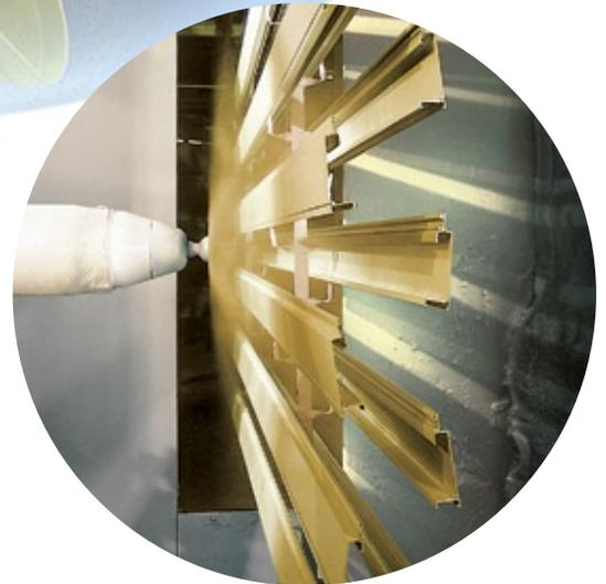
*Nordson electrostatic spray systems and technology provide reliable, accurate performance in all extrusion applications for attractive, durable, quality finishes needed for window and door manufacturing.*
