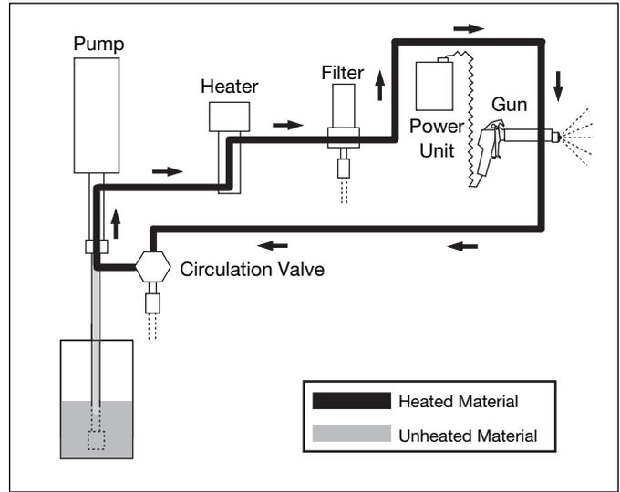
**Heated Airless Electrostatic System**
