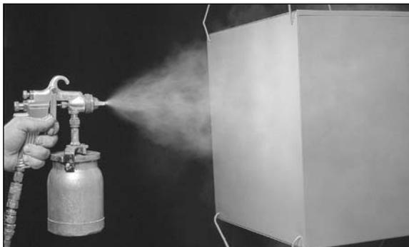
*On external surfaces turbulent air spray creates excessive overspray and high material waste.*
