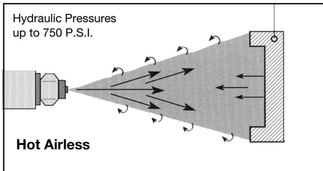
*As heat is applied, solvent vapor pressure increases so atomizing pressure can be reduced. Lower pressure results in lower particle velocity and a softer spray. Better coating coverage and less solvents improve material savings.*
