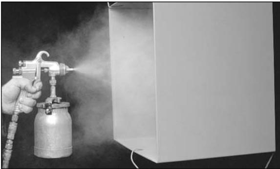
*On internal surfaces particles mixed with air rebound and fail to cover corners and recesses.*
