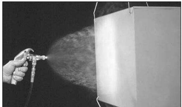
*On external surfaces soft spray creates little or no overspray for minimal waste and cleaner, safer operating environment.*
