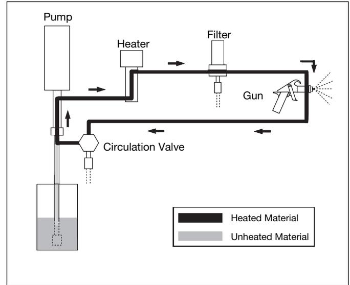
**Heated Airless Circulating System**
