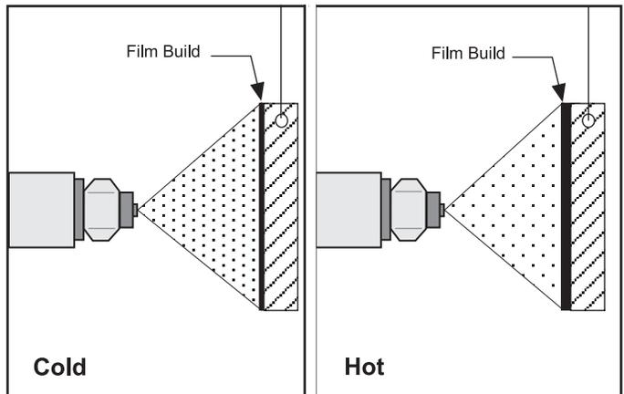
*Heating coatings reduces viscosity and improves sprayability. A higher film build can be applied without sags or runs, and often equals two air-sprayed coats.*
