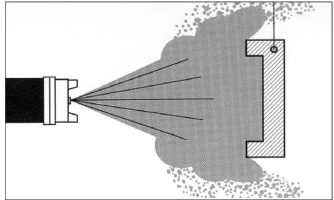
*Conventional air spray creates a "cloud" as high-pressure air jets atomize coatings. As coating particles are blown at high speed toward the part, many are dispersed into the air.*
