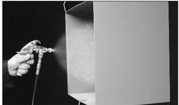
*On internal surfaces no visible bounceback indicates easy-to-control spray for improved first-pass coverage.*
