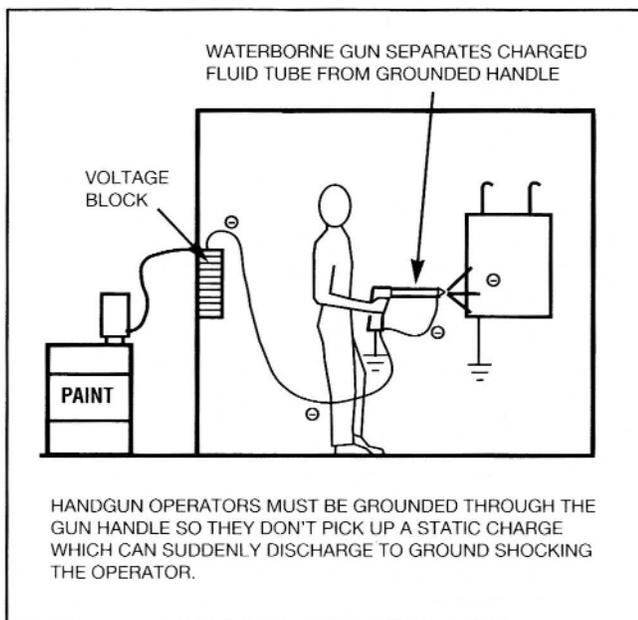
charging" electrodes can charge paint droplets in the air even though there is no direct contact with the paint stream. Any electrical energy that is not drained away from the operator by the grounded gun handle or some other means can accumulate. The electrical energy accumulated in the operator's body this way will eventually short to ground and the sudden release of energy can cause a severe shock and possible injury to the operator.
