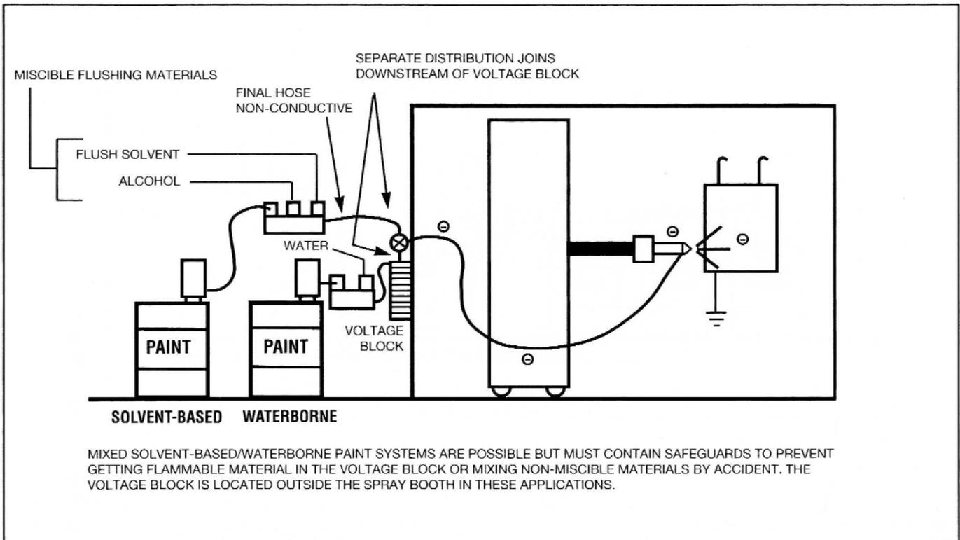
It is possible, however, to design a voltage-blocked application system that uses both waterbornes and solvent-based paints (Fig 3). Here are some design guidelines:
