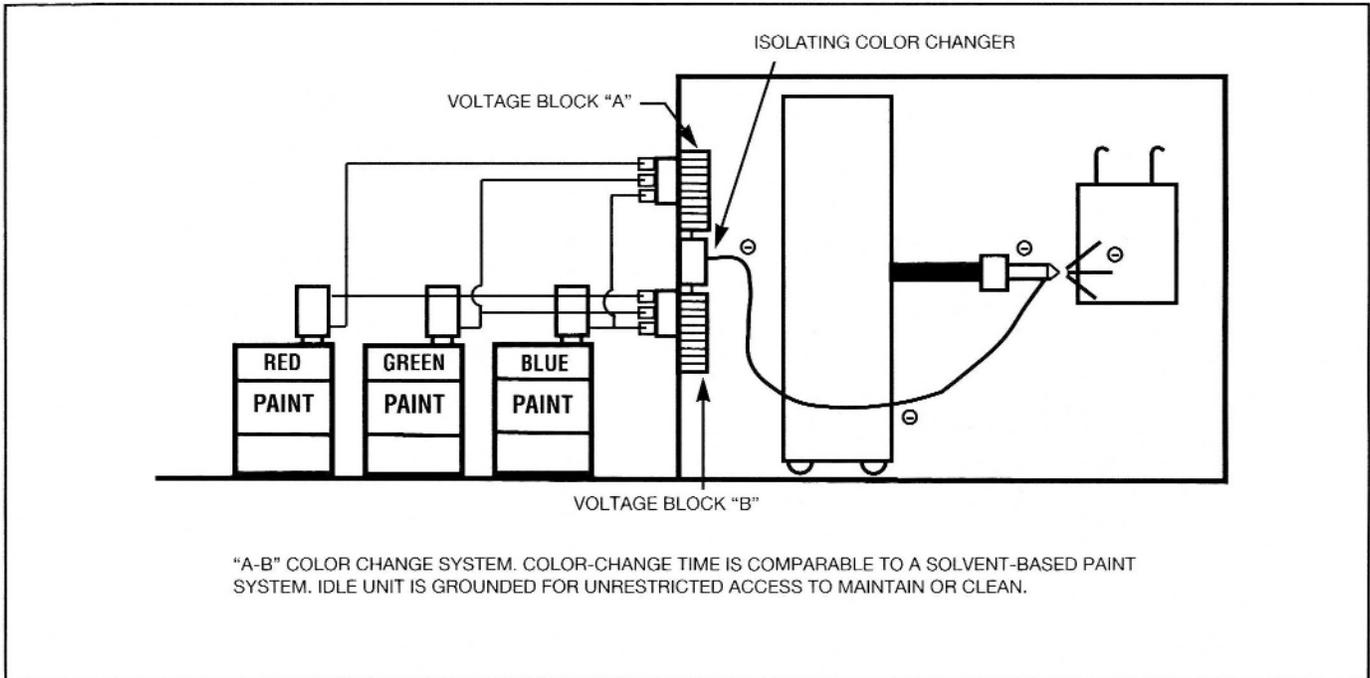
quick connect fluid couplings, all of which need to be cleaned at color-change time. In addition, the voltage block may contain several ounces of the old color paint that will need to be purged out before the cleaning process can begin. A simple voltage-blocked waterborne system can require 5 to 10 minutes for color change.
