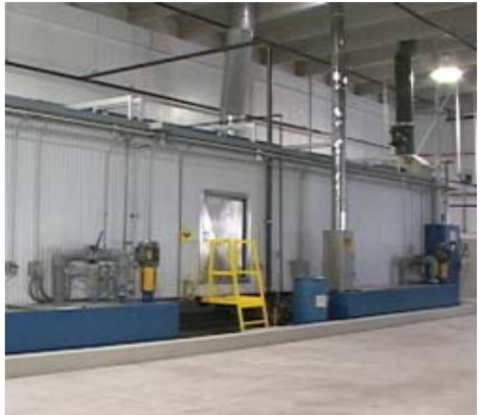
The three-stage washer provides the critical preparation needed for outdoor performance of powder on aluminum. (Photos courtesy of National Partitions)
