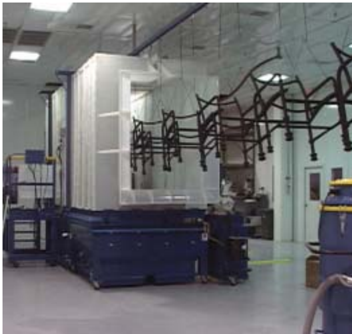
The powder booths are moved off-line for color change.
