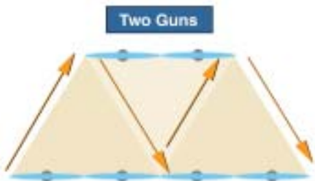
Figure 8. Two Guns Reciprocating Relative to Line Speed
