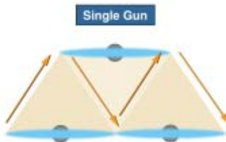
Figure 4. Single Gun Oscillation Relative to Line Speed
