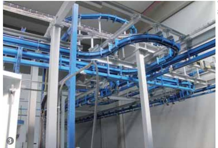
**Figure 3: Detail of the two-rail conveyor system from Futura Convogliatori Aerei.**
