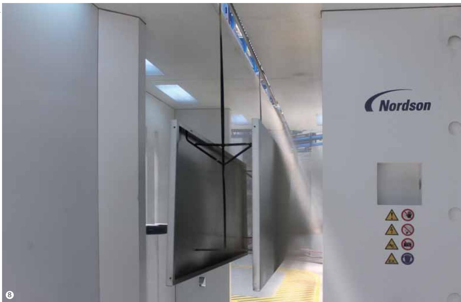
**Figure 8: Application of the coating powder using Nordson Encore HD guns.**
