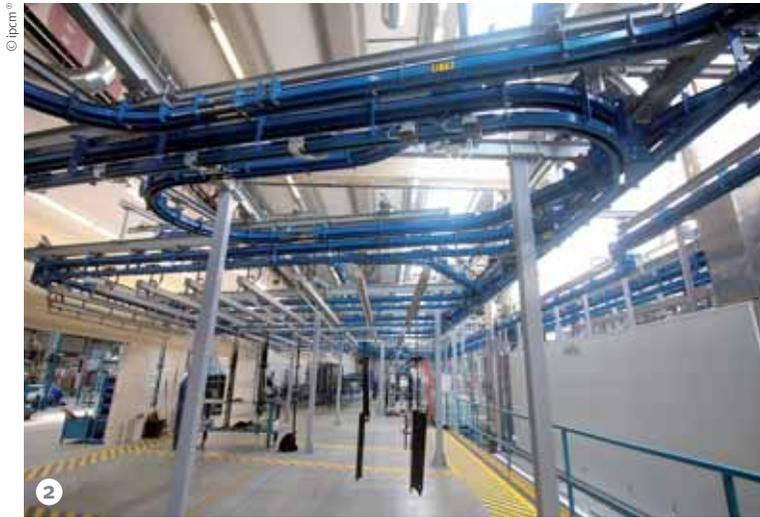
**Figure 2: The two-rail conveyor system from Futura Convogliatori Aerei.**
