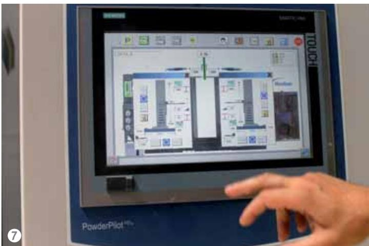
Figure 7: The PowderPilot HD with command touch screen from Nordson's HDLV system.
