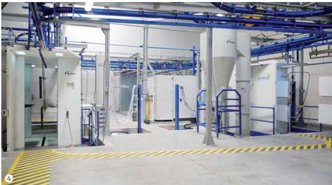
**Figure 4: The twin Nordson ColorMax 3 powder coating booths in parallel.**
