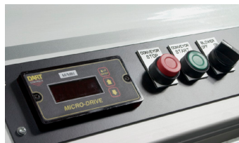
Simple Controls (left), Closed-loop Speed Control, Belt Break Detection (right)
