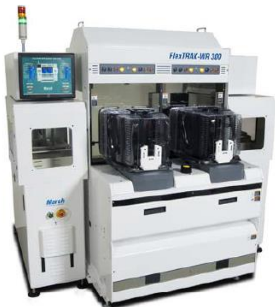
Figure 1. Example of a commercially-available RF plasma system for removing Fluorine, organic and metal oxide contamination from semiconductor wafers using Argon-based (dry) plasma.
