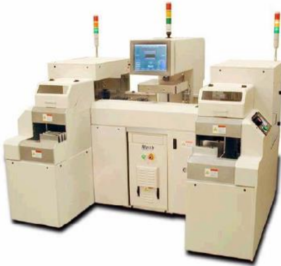
Figure 6. Example of a commercially-available RF plasma system for removing Fluorine, organic and oxide contamination from BGA strips and metal lead frames using Argon-based (dry) plasma.
