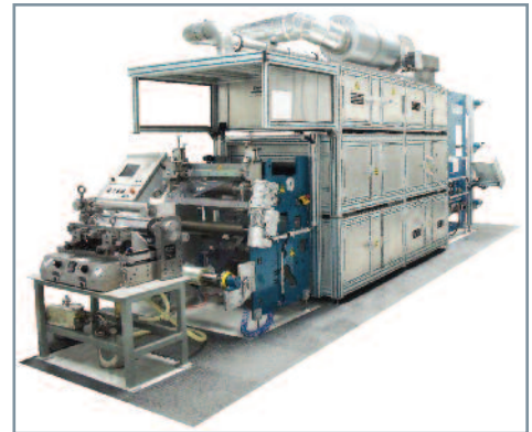
FULLY EQUIPPED—FROM FLUID DELIVERY TO ROLL SYSTEM. Trial lab at Nordson Extrusion Dies Industries facility in Chippewa Falls, WI, U.S.A. is housed in a clean, temperature-controlled room. The coating line has a maximum speed of 60 m/min. and a working width of 500 mm.
