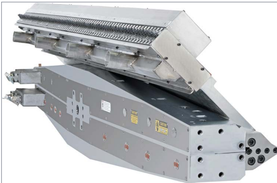
BROADER SCOPE FOR AUTOMATION is available with new-generation gauge profiler on EDI™ Autoflex VI-E die, shown here in rear view with lip exit at bottom right. New lip adjustment system extends obliquely from top of photo to the lip area. Recessed fasteners are visible.
