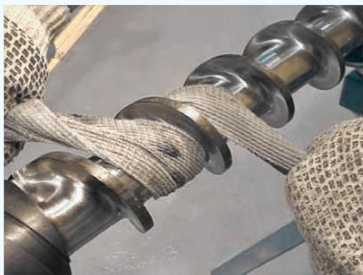
**FIG 4** Final cleaning of the screw channels and flight outside diameters returns the screw to its pristine condition.
