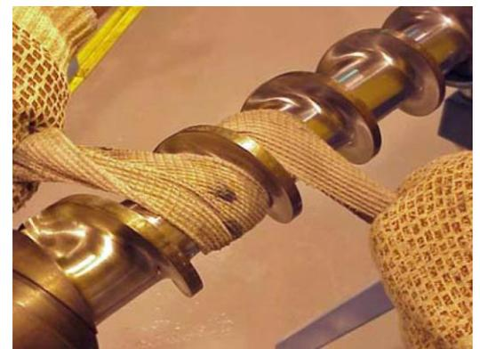
[Figure 4](#). Final cleaning of the screw channels and flight outside diameters returns the screw to its pristine condition.
