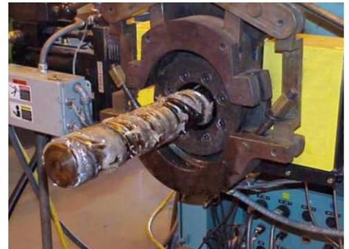
[Figure 2](#). Screw cleaning begins by pushing the screw until the first four or five turns are exposed.
