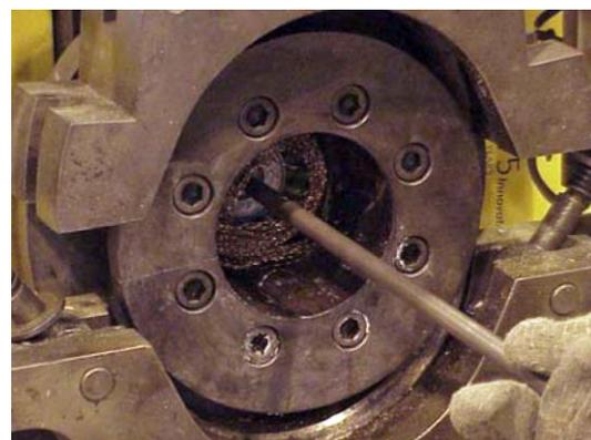
[Figure 6](#). The brush/gauze assembly is pushed into the bore of the barrel.
