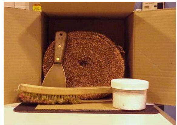
[Figure 1](#). The tools and materials for screw and barrel cleaning are few and simple.
