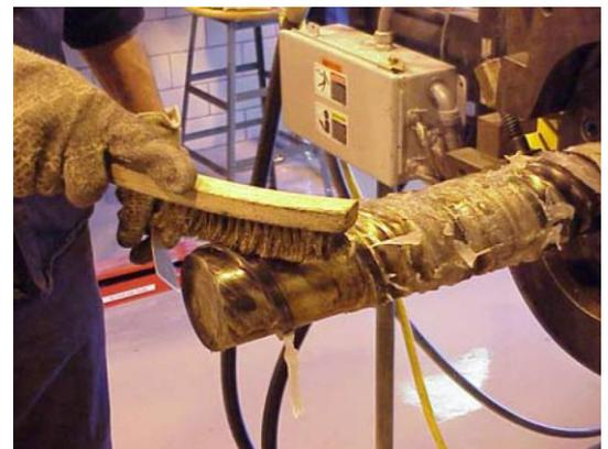
[Figure 3](#). Use a brass wire brush to clean away the purging resins from the screw channels.
