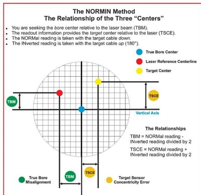
In the NORMIN method of laser alignment developed by Hamar Laser®, a laser that has been aligned with the gearbox axis of rotation is projected onto a two-axis self-centering target that is placed inside the extruder barrel.
