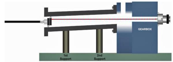
Schematic shows misalignment of the free end of the barrel with respect to the gearbox axis of rotation.
