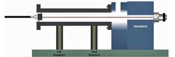
Following alignment, the barrel is fully concentric with the gearbox axis of rotation.
