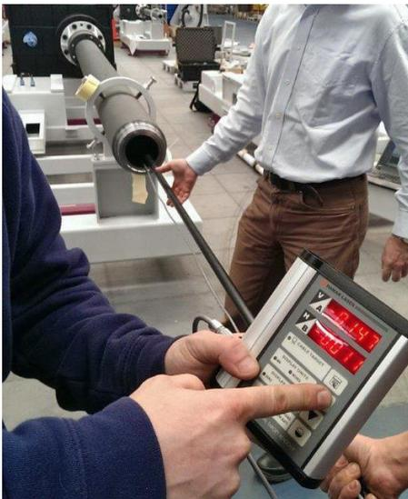
During laser alignment, a pole with the NORMIN target is inserted into the barrel. In the foreground is the digital readout of data from the target.
