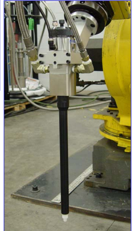
2200-595 Valve and End-Of-Arm Tooling Mounted on Robot Wrist
