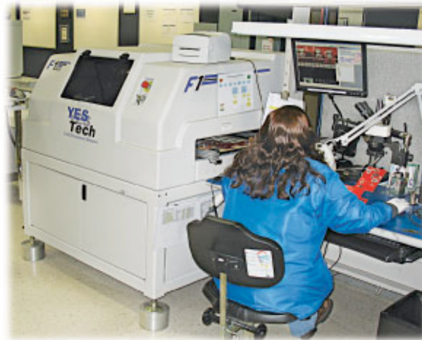
Biamp Surface-Mount Assembly With AOI Inspection
